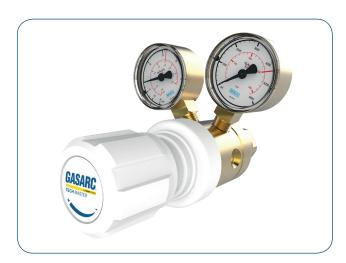
The Tech Master GPT400 Series two stage diaphragm cylinder regulators are designed for primary pressure gas control of of non-corrosive or toxic, technical gases up to grade 4.5 purity (99.995%), on applications where constant delivery pressure is required as the cylinder pressure decreases.
