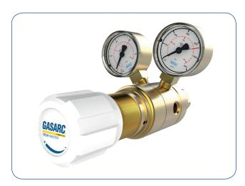
The Tech Master GPT420 Series two stage piston cylinder regulators are designed for primary pressure gas control of non-corrosive or toxic, technical gases up to grade 4.5 purity (99.995%), on applications where constant delivery pressure is required as the cylinder pressure decreases.
