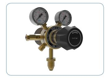
The Tech Master GA600 Series two stage piston cylinder regulators are designed for the primary control of non-corrosive or toxic, technical grade gases up to grade 4.5 purity (99.995%), on high flow, high pressure applications where constant delivery pressure is required as the cylinder pressure decreases.
