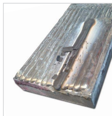
The second FOXcore 347L H-T0 layer shows slag removal similar to that of the first layer.
