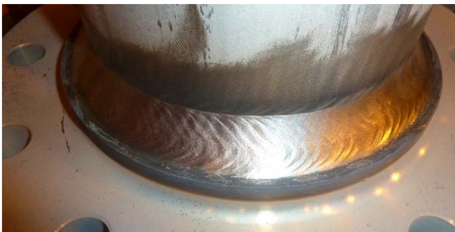
Fillet weld in flat position (PB / 2F). The base material is AISI 304L and the filler FOXcore 308L-T0 DG. Ø 1.2 mm.
