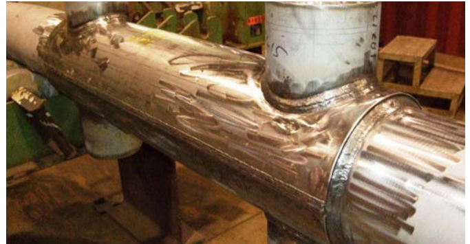
Water injection risers in PUQ jackets. Superduplex welded with FOXcore 2594-T1 HD.
