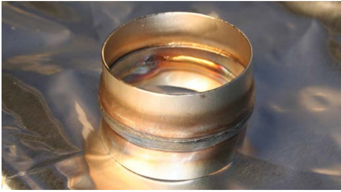
0.6 mm exhaust manifold welded with Ø 1.2 mm FOXcore 308L-MC. With 2.6 m/min wire feeding, 80–85 A and 20 V, the travel speed was 85 cm/min. It was not possible to use solid wire for this sheet metal application.
