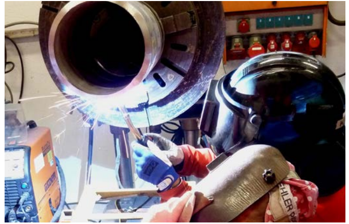
Welding of superduplex UNS S32750 pipe, using FOXcore 2594-T1 HD.
