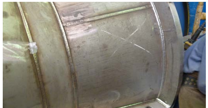
Seawater pump in UNS S32205 duplex stainless steel welded with FOXcore 2594-T1 for highest possible corrosion resistance.
