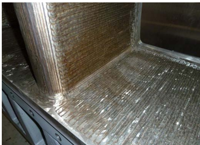
Cladding using FOXcore 309L-T1 for high surface quality, also when welding out of position.
