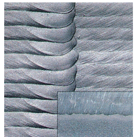
Cladding with FOXcore 309L Mo-T0 and FOXcore 316L-T0 for the 2 nd layer. Results in very uniform ferrite levels.
