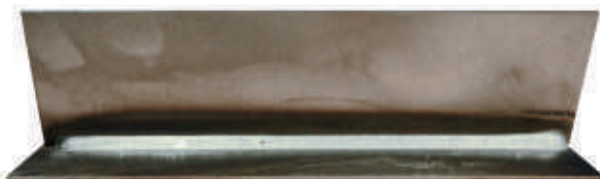
Fillet weld 2.0mm plate in Ar/8% CO 2 shielding gas. 20cm length.
