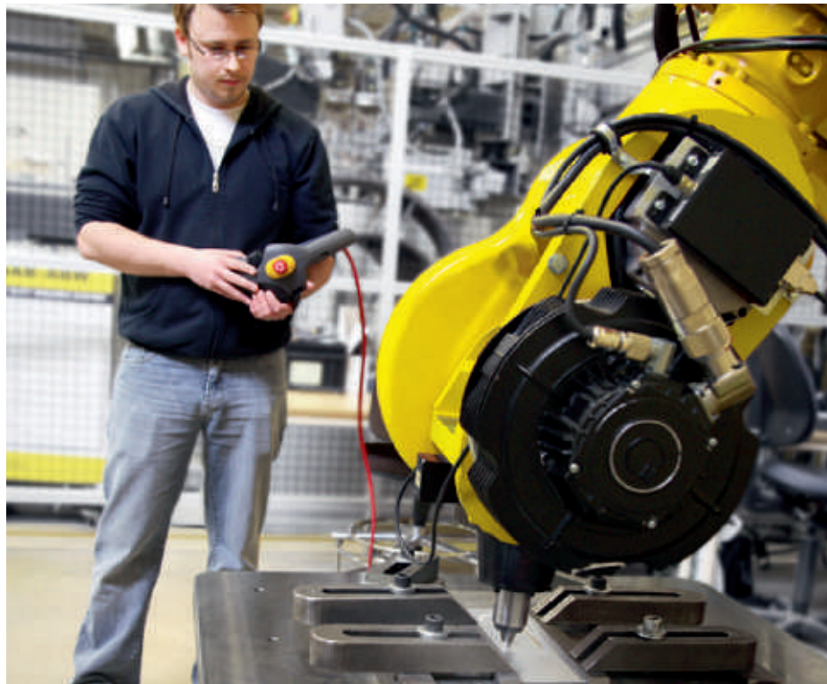
Figure 1. Welding tests on Rosio™ Friction Stir Welding robot.
