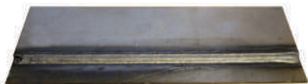
Overlap weld 2.0mm plate in Ar/8% CO 2 shielding gas. 20cm length.
