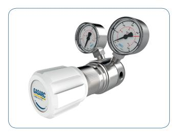
The Chem Master SGS620 single stage piston cylinder regulators are designed for primary pressure gas control of corrosive, toxic and high purity gases up to grade 6.0 purity (99.9999%), on applications where slight pressure variation from decreasing cylinder pressure is acceptable.
