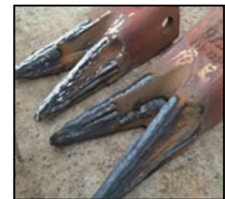
Stoody Vancar applied to excavation teeth.
