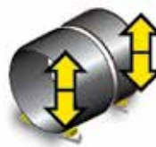
Joining of shell sections using roller beds with hydraulic fit-up system. Internal and external submerged-arc welding performed by a column and boom station.
