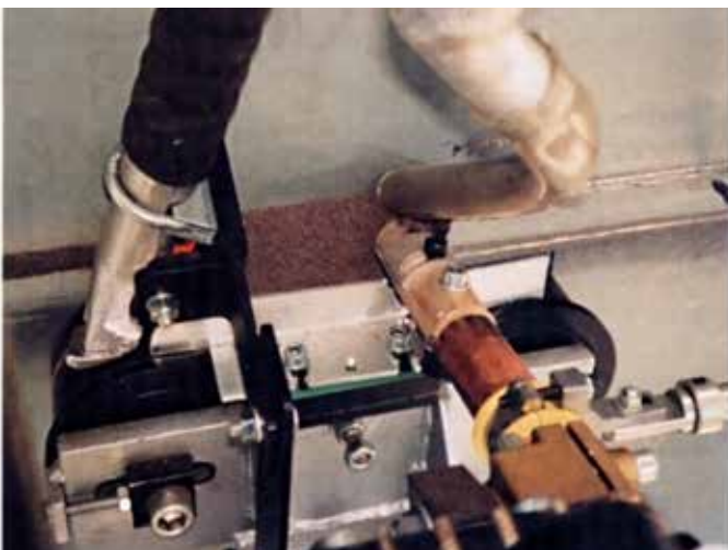
Close-up of the welding head.
