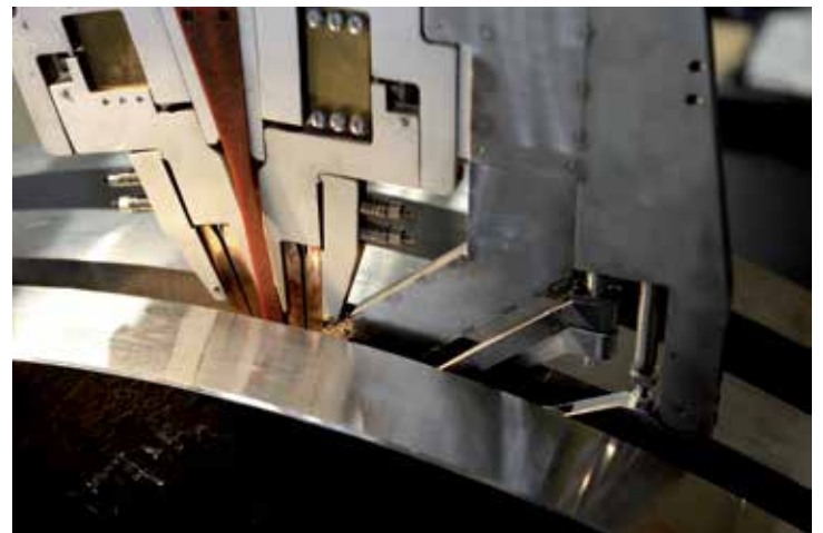
Double-sided joint tracking
