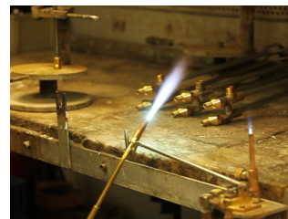
Fluent adjustment of the flame
