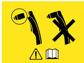
Figure 5.17 - Torch or consumables installation error screen
