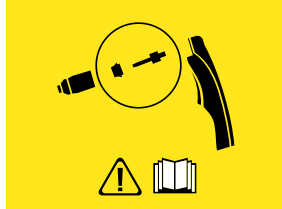
Figure 5.18 - Electrode or cutting nozzle installation error screen
