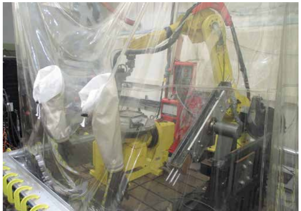
Flexible Welding Enclosure® for Titanium Additive Manufacturing
