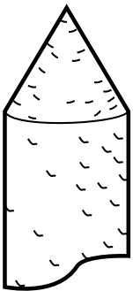
2% Thoriated Tungsten showing risk of uneven thoria distribution
