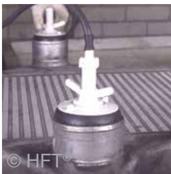
Hollow shaft plugs being prepared for testing an intercooler
