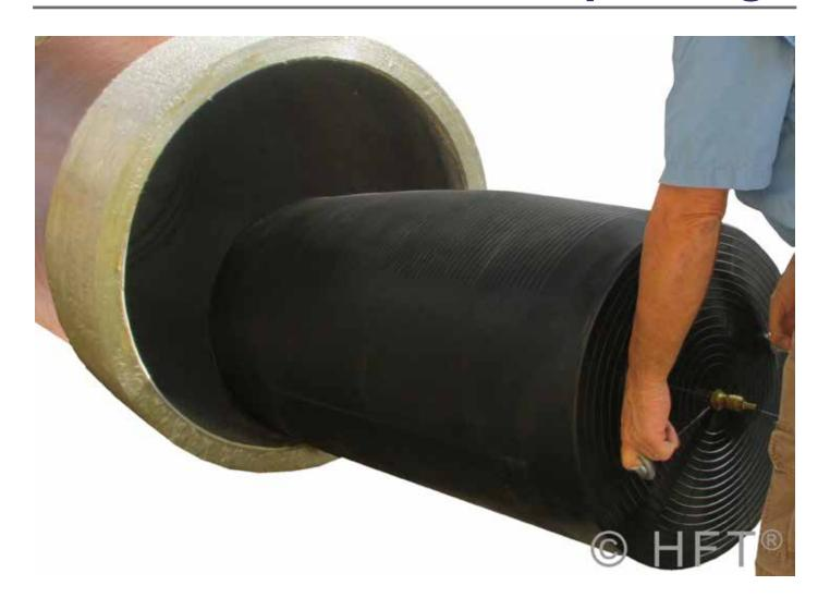
The Pipestoppers® Division Huntingdon HFT®'s **Techniques** Fusion Inflatable Rubber **Plugs** cover а range 2" - 78" (51 to 1,981 mm), each having a wide degree of flexibility in diameter (see chart overleaf). They can withstand a temperature from -40 to +70°C, suitable for use in petrochemical applications, as well as many others, some of which are shown in the next column.
