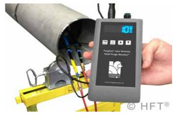
Portable 'handy' Weld Purge Monitor® to read from 1000 ppm down to 1 ppm, accurate to 10 ppm.
