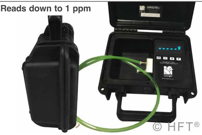
The **PurgEye® 1500 Site IP68** is a portable, 1ppm Oxygen Weld Purge Monitor® integrated into a robust case. Specifically designed for use in rugged site conditions.
