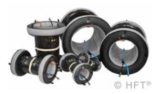
**Argweld® QuickPurge®** Systems are used for larger diameter, high quality, reliable welding of stainless steels, duplex steels and titanium tube and pipe joints to ensure a very fast weld purge time and a very high quality weld root, free from oxidation and discolouration.
