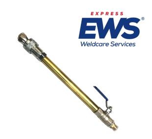
The brass body of the holder is fitted with a 3/8"BSP nipple for connection to the oxygen supply, a ballvalve for control of oxygen, and a quick release carrier to which the required size probe for your lance is fitted.
