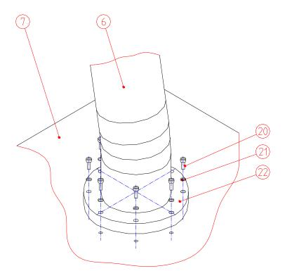
The extractor fitting (e.g. an extractor hose or an extractor arm) must be mounted on the extractor spouts or the housing cover.
