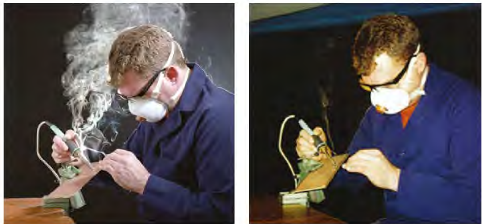
Figure 45 Soldering with and without Tyndall illumination
