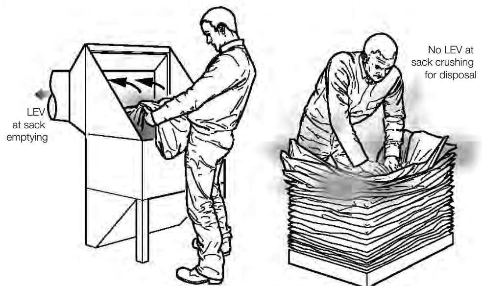
Figure 6 An LEV system to control dust from sack emptying but uncontrolled sack disposal
