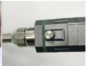
6. Put the protective mirror into the protective mirror holder, push it into the protective mirror holder cavity, and tighten the screws
