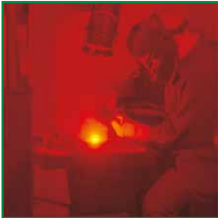
Orange: Shielding during arc welding
