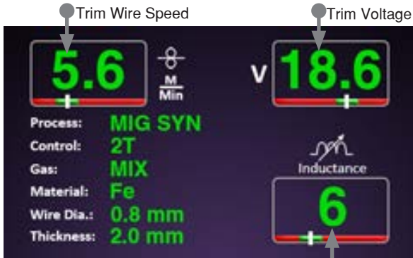
Adjust Inductance (short circuit current)
