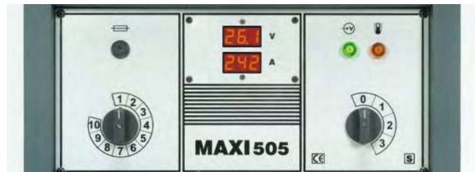
CONTROL PANEL Digital ammeter/voltmeter with hold function of the last welding parameters ( optional )
