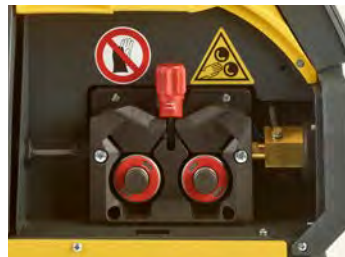
Professional double groove feeding mechanism with 4 rolls
