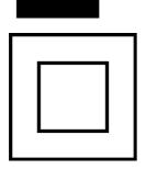
All the electronics in this equipment are double insulated.
