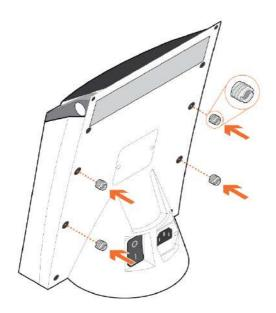
2. It is very important that the slot on the insert is facing out so the insert can be unscrewed for servicing the device
