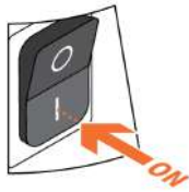
Figure 11 - Power switch in the ON position
